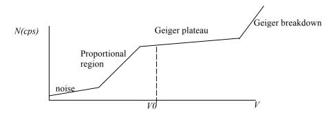
With a Cs-137 or Th-204 βeta source Record N counts for 30s each at voltages 300-1200 V.
